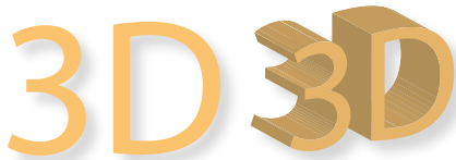
Extruding an object using the Effect > 3D > Extrude & Bevel dialog—the two-dimensional object on the left was extruded to create the three-dimensional version
